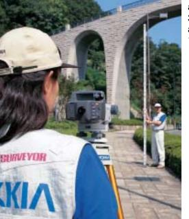
The POWERLEVEL SDL: memory: combining user-f with unprecedented cost pe identifies staff attitude and indicates in negative (-) values. The maximum length of the RAB Code Staff is 5.0m (16.7 ft.) facilitating survey work where there are steep slopes.
